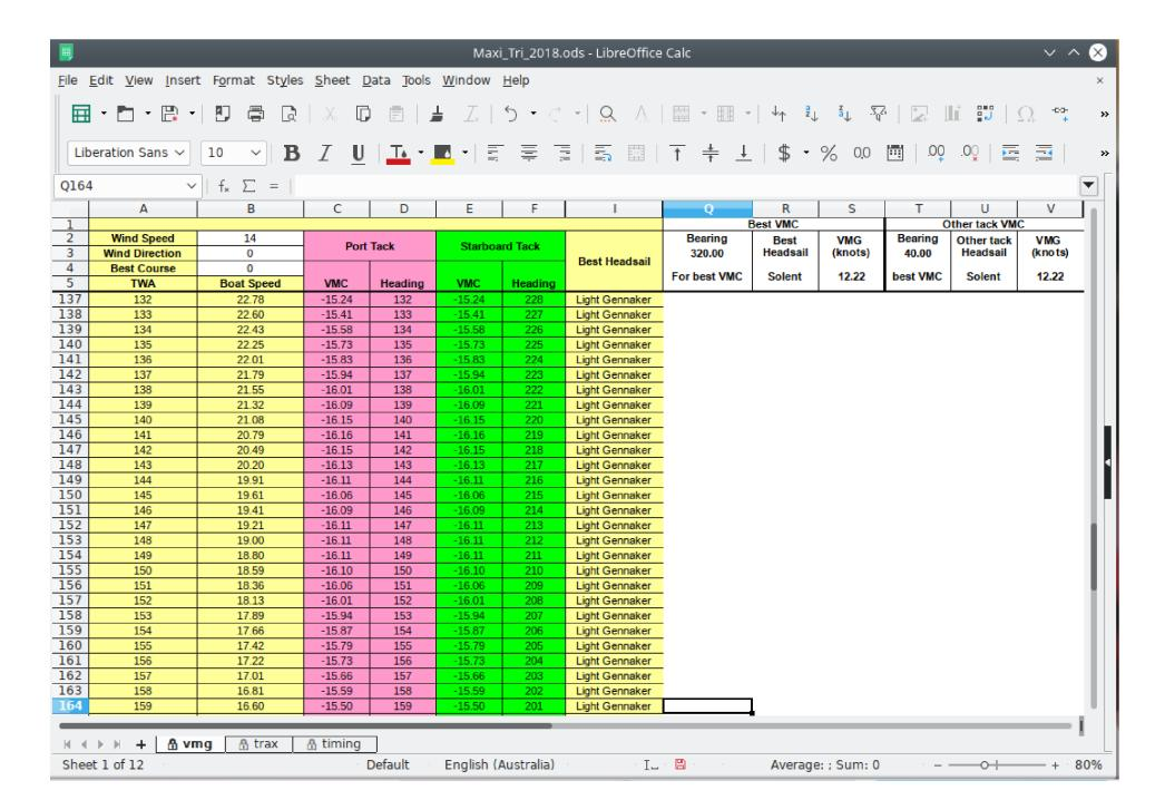
In cell B2, enter the wind speed, don't forget to round up or down as RG does, the calculator works quite well with decimals but RG can't do it yet.
