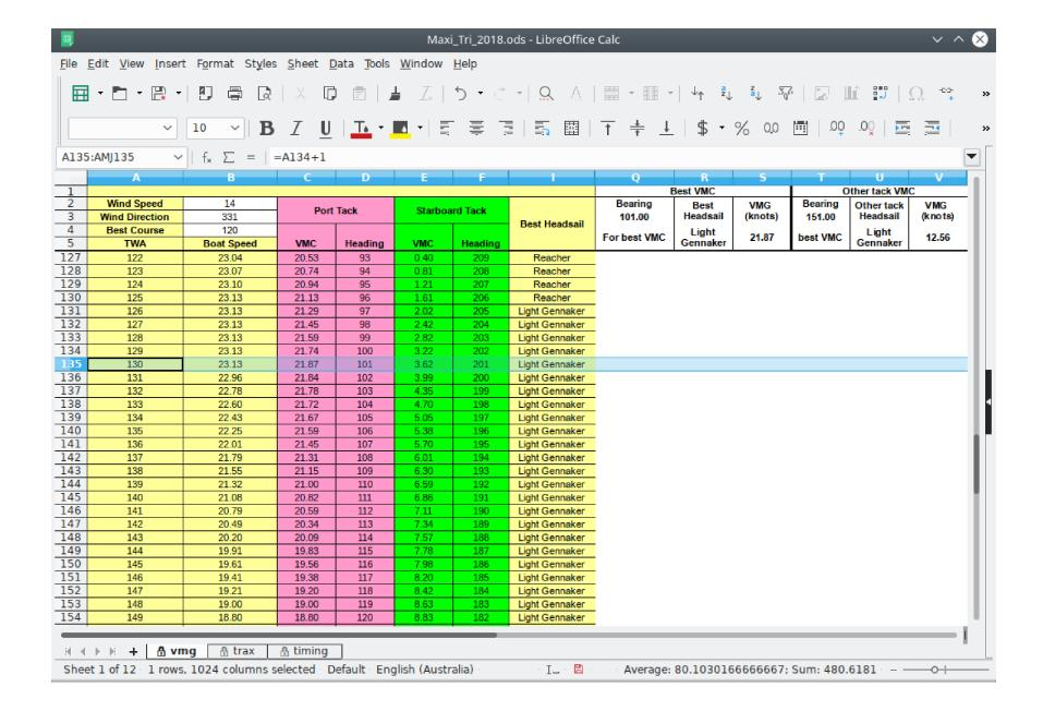
So the best heading to reduce the distance in the direction 120 is 101, the sail to use is the light gennaker, the boat speed is 23.13 knots but the VMC is 21.87 knots. On the other hand, with the same TWA on starboard tack, the VMC is only 3.62 knots.
