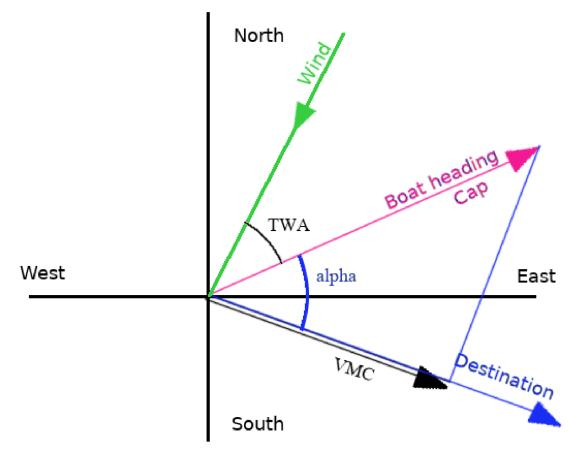
VMC is derived with a formula similar to that of the VMG, but with alpha instead of TWA as angle:
